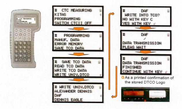
**Please Note** that if you load more than one OEM variant parameter set, the display may indicate 'ERROR, TCO – NEG. RESPONSE'. To start the process of reprogramming a further OEM parameter, program the DTCO back to 'VDO UNIVERSAL' (i.e. factory re-set)
